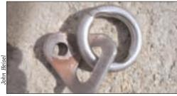
This anchor is less than four years old. Half of the steel was worn away, resulting in a safety hazard.
