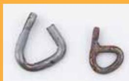
water out—or so they thought. In fact, it sometimes did the opposite by trapping moisture in the hole, as rock is porous and water can still work its way to the bolt. In those cases, the water just had a harder time leaving, creating unsafe bolts sooner than may have otherwise happened.
